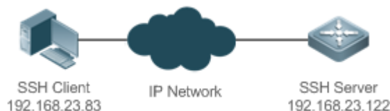
Figure 8-5 Networking Topology of SSH File Transfer
