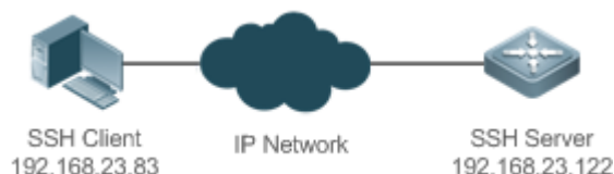
Figure 8-1 Networking Topology of SSH Device Management
